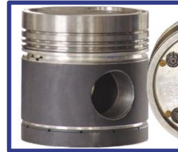
Al piston with steel FERROTERM insert
